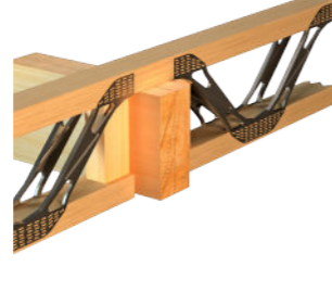
SD7 - Internal Bearing Pocket
